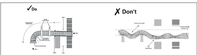
The inner radius of any bend should be greater or equal to the diameter of the ducting being used. If the radius is reduced, the resistance of the bend will increase and the volume of the air being extracted will decrease (image on the left)
